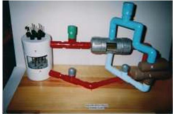
For simplicity, I only show one “loop” and only some of the absolute components (steam drum, pressurizer/de-gassifier, boiler, turbine, condenser, and primary and secondary pumps). Using the model made of PVC piping and connectors is much better than just simplified pictures in a book.
